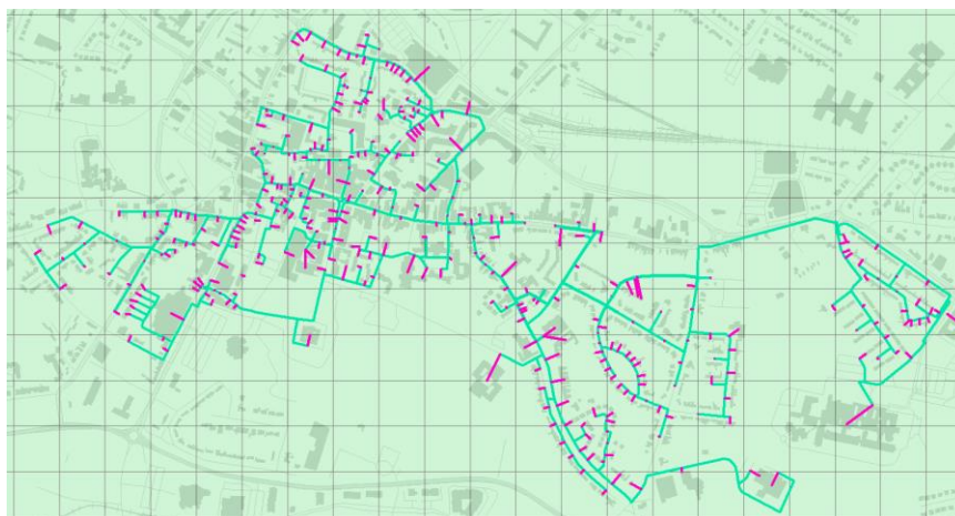
Figure 4: Initial design Tralee town centre district heating, based on OPTIT simulations. Source: OPTIT, 2017.
